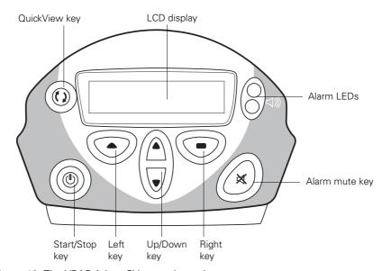
Figure 13: The VPAP Adapt SV control panel
